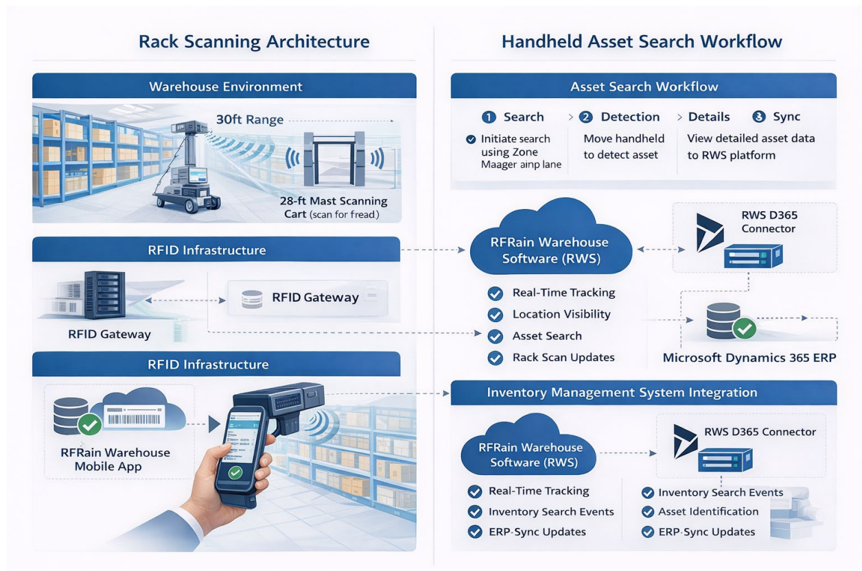
Figure 2 – Rack Scanning Architecture and Handheld Asset Search Workflow
